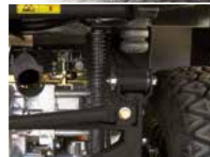
Robust, reliable semi-independent rear suspension
