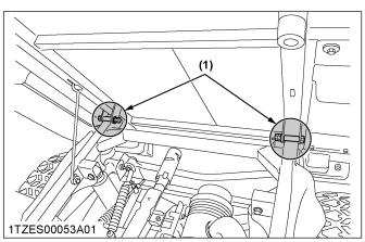
(1) Cargo bed pivot (spray type grease)
