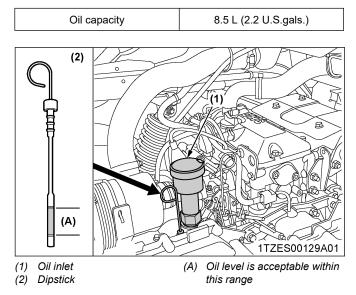
6. After running the engine for a few minutes, stop the engine and check the oil level again; add oil to prescribed level.
