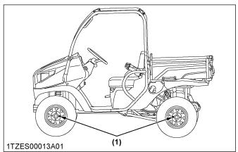
Torque wheel bolts to 108.4 to 121.9 N m (11 to 12.4 kgf m) (80 to 90 lbf ft) Aluminum wheel:130 to 150 N m (13.3 to 15.2 kgf m) (95.9 to 110 lbf ft)
