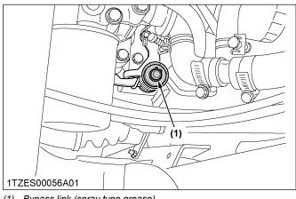
(1) Bypass link (spray type grease)
