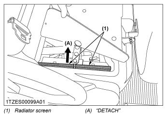
3. When you put it back, push in the screen to the protrusion.
