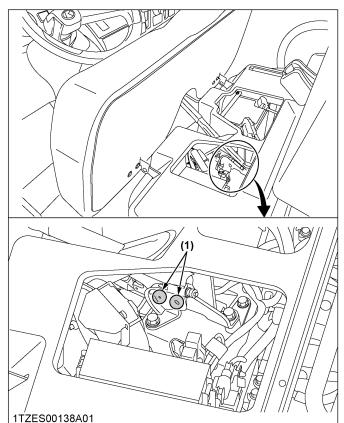
(1) Parking brake lever pivot (spray type grease)
