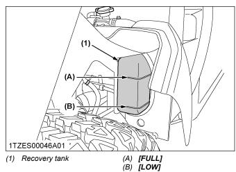
3. When the coolant level drops due to evaporation, add water only up to the full level. In case of leakage, add antifreeze and water in the specified mixing ratio up to the full level.
