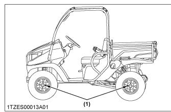
(1) Torque wheel bolts to 108.4 to 121.9 N ⋅m (11 to 12.4 kgf ⋅m) (80 to 90 lbf ⋅ft)
