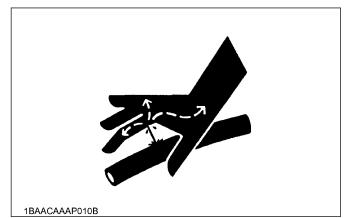
Fluid escaping from pinholes may be invisible. Do not use hands to search for suspected leaks; use a piece of cardboard or wood. Use of safety goggles or other eye protection is also highly recommended. If injured by escaping fluid, see a medical doctor at once. This fluid will produce gangrene or severe allergic reaction.
