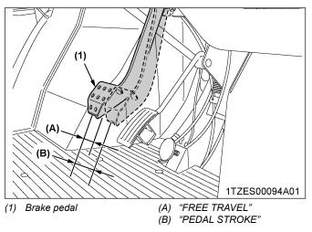
3. If brake pedal free travel is outside of the specifications, contact your local KUBOTA Dealer for adjusting the brake.
