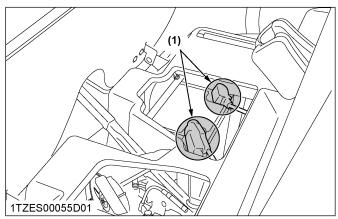
(1) Battery terminals (spray type grease)
