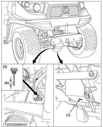
(1) Drain plug(2) Filling plug with dipstick
