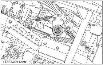
(1) VHT link (grease fitting)
